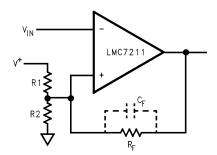
$R_F \gg R_1$  and  $R_F \gg R_2$
