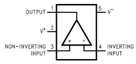
Figure 2. 5-Pin SOT23-5 **Top View**
