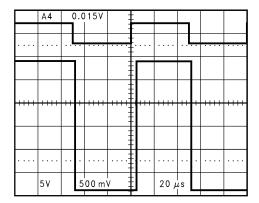
Figure 3. Even at Low-Supply Voltage of 2.7V, an Input Signal which Exceeds the Supply Voltages
