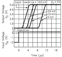
Input Overdrive Referenced to  $V_{OS}$
