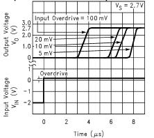
Input Overdrive Referenced to  $V_{OS}$
