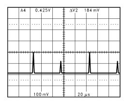
Figure 5. Measurement of the Shoot-Through Current
