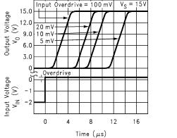
Input Overdrive Referenced to  $V_{OS}$
