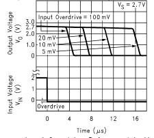
Input Overdrive Referenced to  $V_{OS}$
